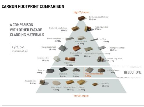
The Construction Material Pyramid was developed by the Centre for Industrialised Architecture (CINARK) at the Royal Danish Academy in 2019. It is a way of visualising the carbon emissions associated with the production of different materials. The pyramid focuses on the product stage (life cycle phases A1 - A3). It gives an impression of the global warming potential of fibre-cement boards in general compared to other cladding materials.
