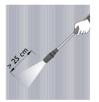
When high pressure cleaners with warm water are used a maximum pressure of 20-30 bar for coated panels, and 80 bar for uncoated panels is advised. For cold water devices a maximum pressure of 20-30 bar for coated panels, and 100 bar for uncoated panels is admitted. Use of rotating nozzles is not allowed. The maximum flow rate is always 10 litres/minute.
