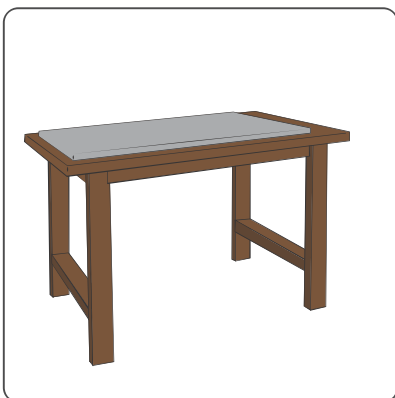
Stable Work Table With Sacrificial Board/Fibre Cement
