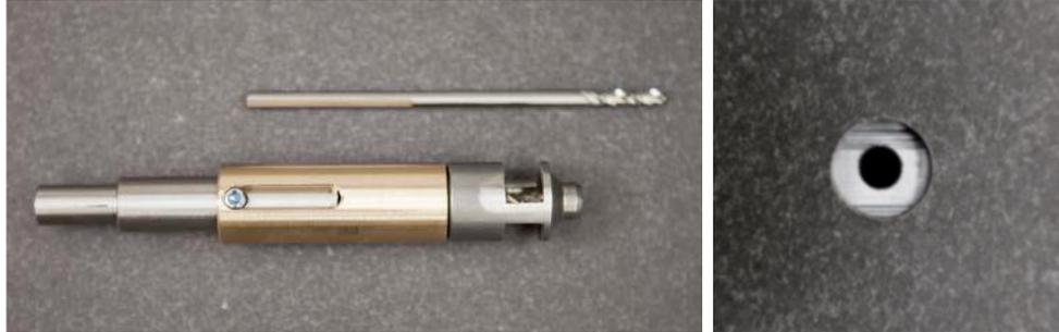
The centralizing tool has a guide that neatly fits into the panel hole. When depressed, the tool extends the small drill bit to drill the metal rail.
