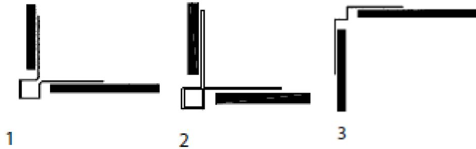
The profiles should be butt joints and should never overlap.
