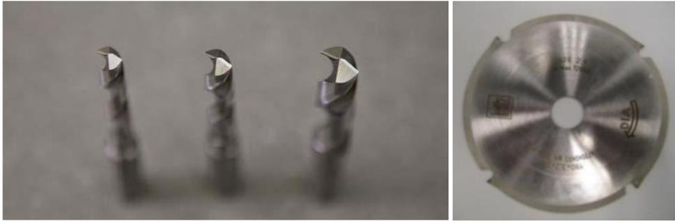
Saws, or handsaws, used to cut EQUITONE panels should be capable of 4000-6000 RPM. Ensure the direction of the blade rotation allows the leading edge of the blade to cut into the face of the panel. This prevents chipping of the panel face. Saws with guide rails and vacuum systems are highly recommended. Festo and Mafell brands are recommended.
