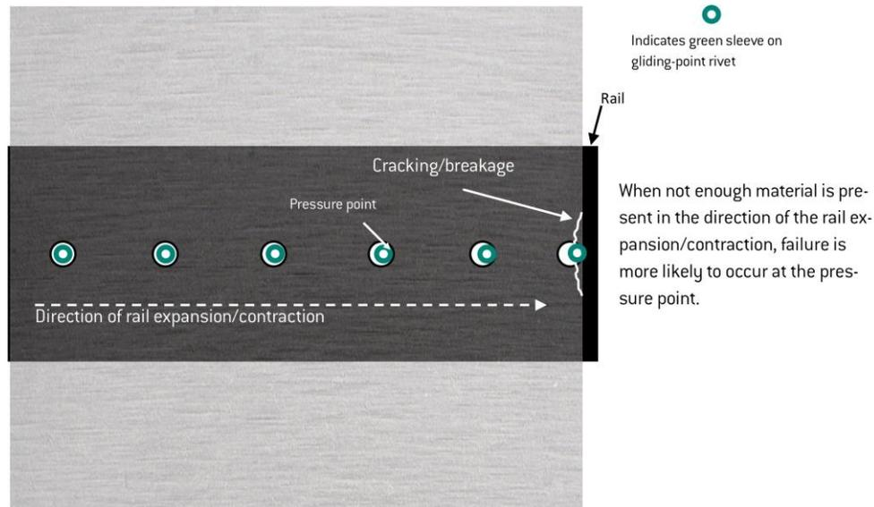
The above illustration shows how the gliding-point rivets can move, contact the panel, and potentially cause cracking/breakage as a result of the pressure exerted if less than 2 - 3/4" spacing was used. Having a minimum of 2 - 3/4" spacing from the edge rivet to the edge of the panel should significantly reduce the likelihood of occurrence as there is enough material left to resist the pressure. Here is the edge spacing:
