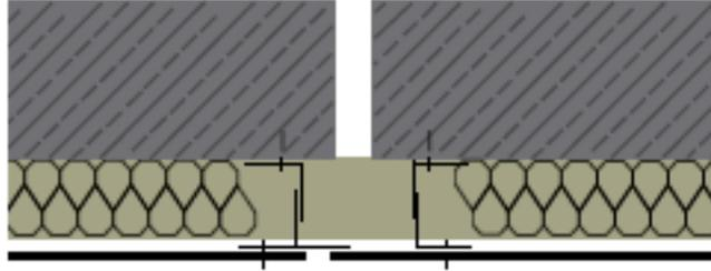
Coordinate vertical joints in façade panels with the position of the expansion/movement joint. An additional profile is used to support one of the panels. An adjustable “T” profile may be used, which allows the panel to slide.
