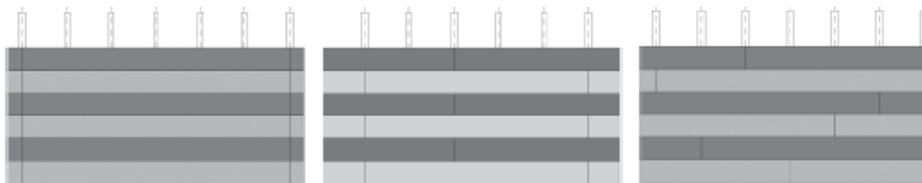
The size of the holes to be drilled in the plank is the same as large panels. Note, all fasteners, whether rivet or screw, must be at  $90^\circ$  to the plank. Adhesive and Tergo+ mechanical fasteners are not possible with this arrangement.
